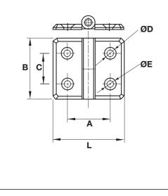
**1-243-6074 (S)** R/H 40x40 **1-243-6073 (S)** L/H 40x40 To hinge size 40 (lift off type see example page 37)
