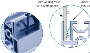
Panel retaining clip, min\_3 off/metre
