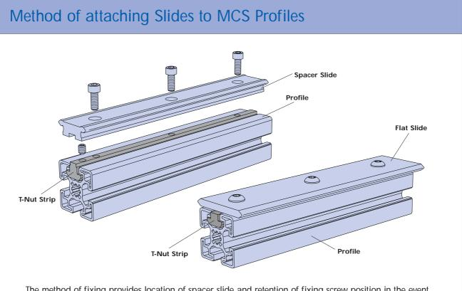
The method of fixing provides location of spacer slide and retention of fixing screw position in the event of disassembly.
