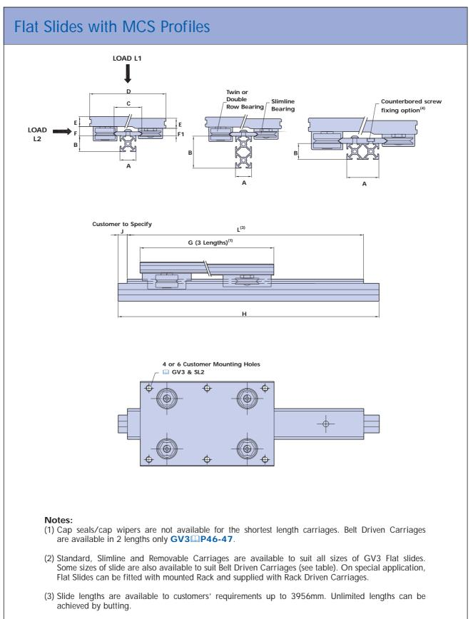
(4) The counterbored screw fixing option with low head socket cap screws DIN 6912 will be supplied for double row slide fixing when used with slimline carriage.
